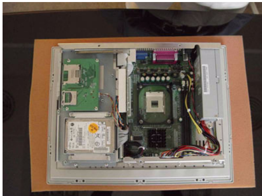
Figure 4.4: The PPC without the Rear Cover
